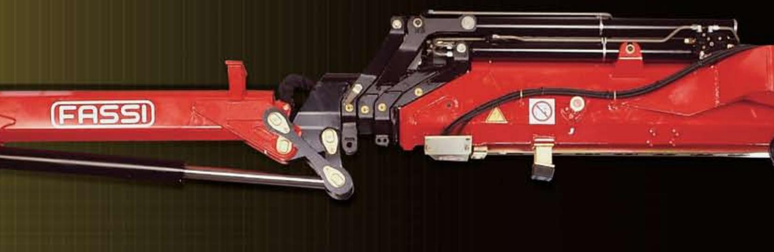
to reduce the encumbrance height of the jib itself. The result has been achieved by fitting the rams to the sides of the jib.
