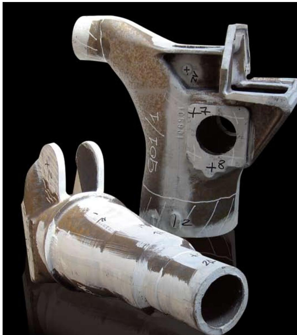
*These pictures show two cast enbloc base and column elements after checking: the lighter areas indicate the dimensional tests performed by tracing, the points that are highlighted are the areas subjected to X-ray analysis. These controls make it possible to check compliance of the dimensions and identify possible internal faults.*
