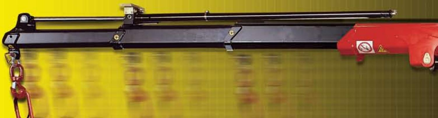
First of all, we must remember that a hydraulic jib is a third boom that can be added to the standard machine using a special coupling device. In view of the importance that these jibs have for operation of a crane, Fassi has dedicated great attention to this element, designing and creating the jibs with the
