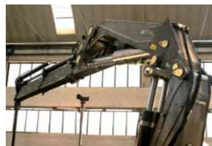
One specific area in Fassi's plant at Albino is entirely dedicated to the various fatigue tests, organised in a number of stations that subject prototypes to the severest possible experimental testing operations.
