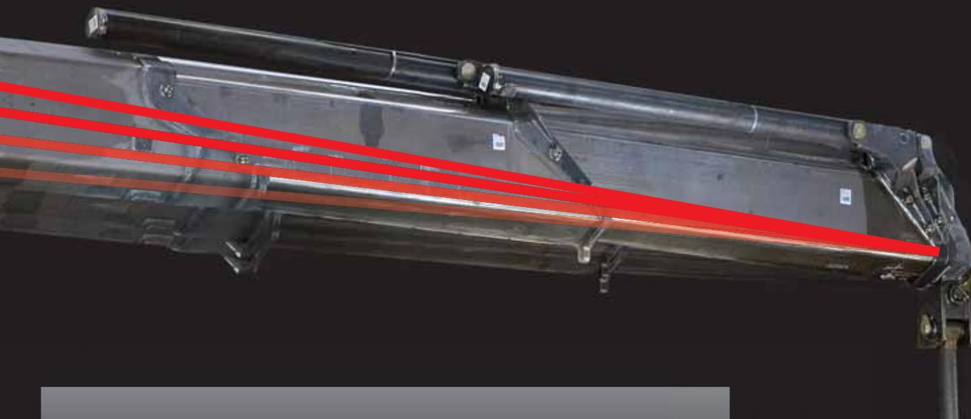
“During fatigue tests we simulate the working conditions the crane will have to face as exactly as possible, so we do not just lift from fixed positions, but we test at various reaches and with various loads at different lengths”.
