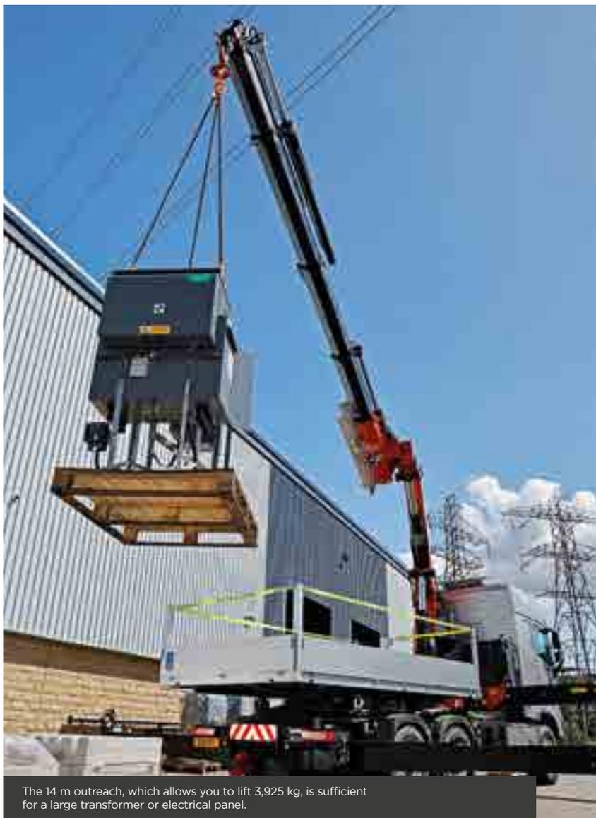
The 14 m outreach, which allows you to lift 3,925 kg, is sufficient for a large transformer or electrical panel.
