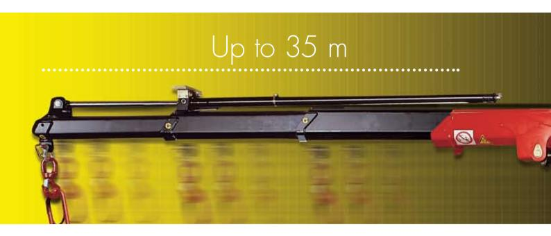
First of all, we must remember that a hydraulic jib is a third boom that can be added to the standard machine using a special coupling device. In view of the importance that these jibs have for operation of a crane, Fassi has dedicated great attention to this element, designing and creating the jibs with the
