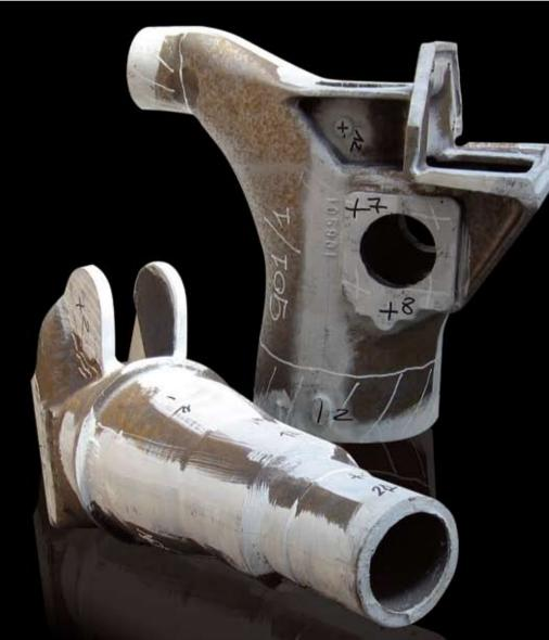
These pictures show two cast enbloc base and column elements after checking: the lighter areas indicate the dimensional tests performed by tracing, the points that are highlighted are the areas subjected to X-ray analysis. These controls make it possible to check compliance of the dimensions and identify possible internal faults.
