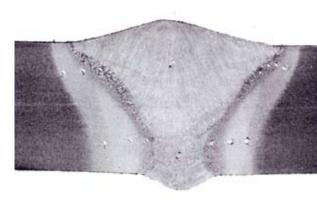
Fassi uses macrography to verify compliance of the welds. In this case it is possible to note two welds that have been correctly performed, and therefore comply with Fassi requirements.
