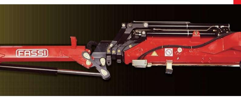
to reduce the encumberment height of the jib itself. The result has been achieved by fitting the rams to the sides of the jib.
