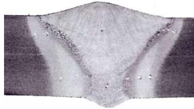
*Fassi uses macrography to verify compliance of the welds. In this case it is possible to note two welds that have been correctly performed, and therefore comply with Fassi requirements.*
