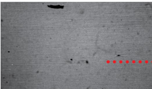
The two micrographies are an example of the scrupulous way in which Fassi checks the quality of materials: it highlights a comparison of the level of inclusions in the steels, deriving from castings in two different supply batches.
