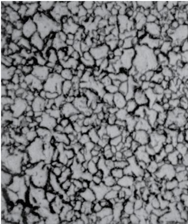
Fassi uses micrographic tests to check the size of the austenitic and ferrous grain of steels, so as to determine the tenacity of the material.
