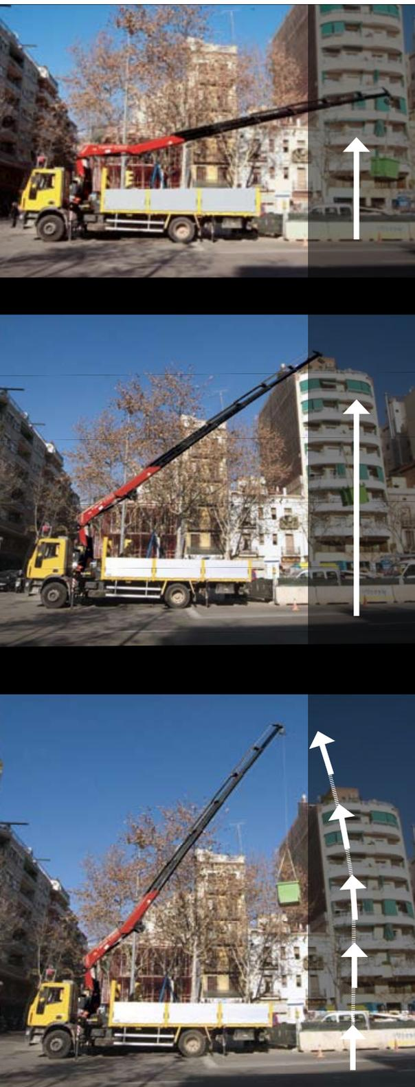
*The considerable results seen during our test have been made possible thanks to a Fassi system known as XF: a new system of lock valves for the lifting rams and oil regeneration valves for the extension rams, which reduces the machine's working times.*
