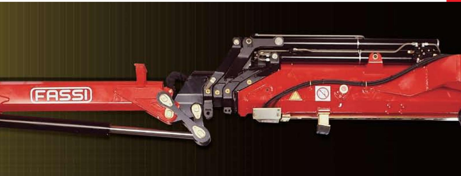
to reduce the encumberment height of the jib itself. The result has been achieved by fitting the rams to the sides of the jib.
