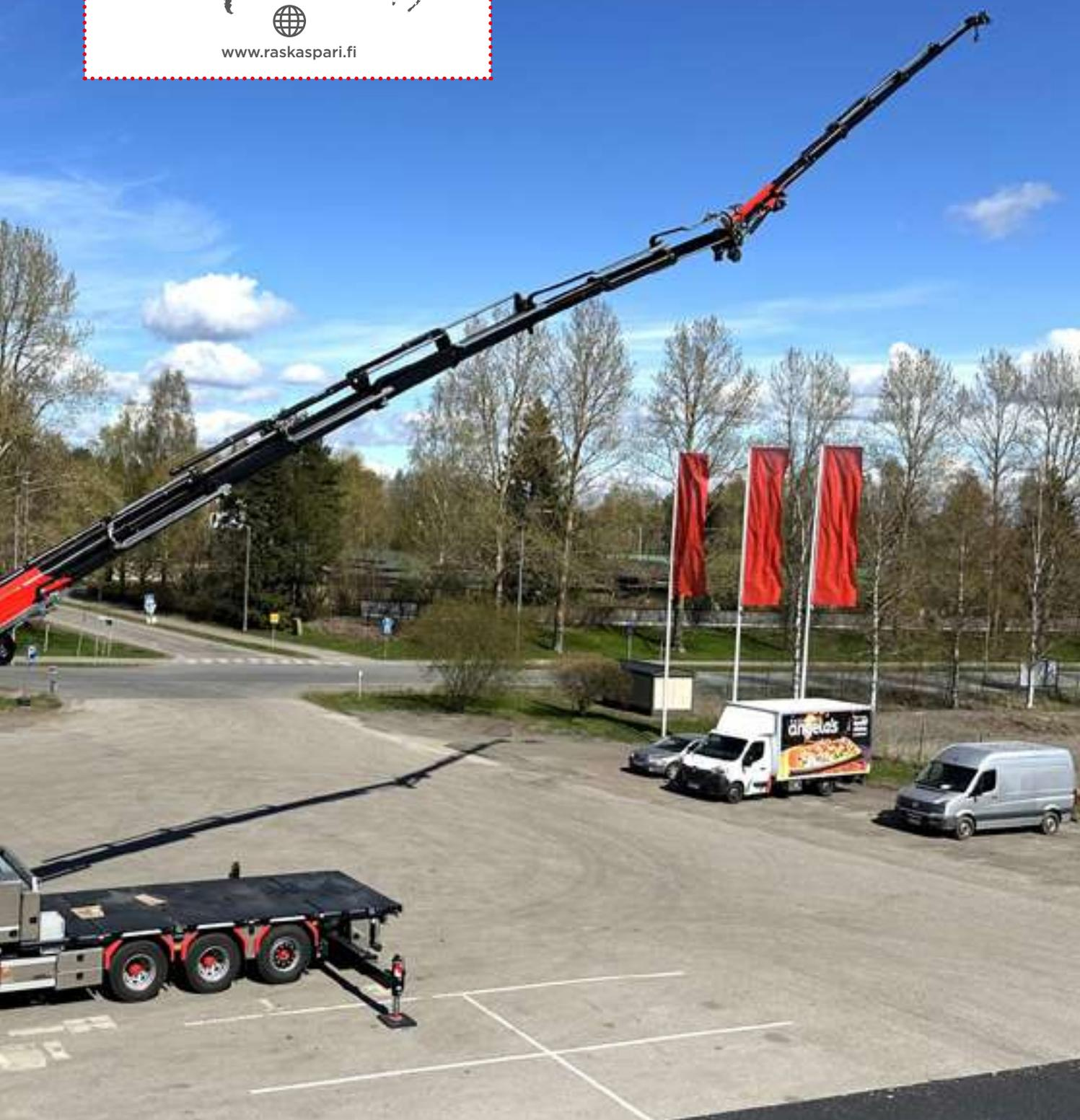
**The Fassi F1250R-HXP, with its nine booms, is the first of its kind in Finland. Weber added: “The nine-extension crane has a horizontal outreach of over 21 metres. It has an excellent power-to-weight ratio and includes advanced features such as FSC TECHNO stability control.”**
