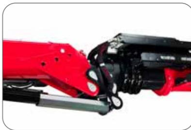
This allows the operator to extend the arms to a height of up to 25.6 metres. This is a great advantage for those working in handling plasterboard panels which, thanks to the F375SE and its 5000 kg weight, can be lifted up to the seventh floor of a building.
