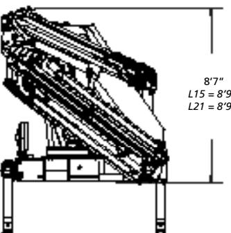
The diagram shows a side profile of the L SERIE F415RA e-dynamic with height dimensions: 8'7", L15 = 8'9", and L21 = 8'9". To the right is a top-down view with dimensions: 8'4", L15 = 8'4", L41 = 8'4", 5'2", 5'8", L15 = 5'5", and L15 = 5'11". Below the drawings is a table comparing L153, L154, L212, L213, L214, L323, L324, and L413 models across three categories: NL (52 lbs), PL (46 lbs), and OL (48 lbs). The table also includes L414 (850 lbs) and NL (70 lbs) values.
