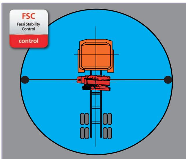
A Fassi system that continuously monitor and ensure the ideal crane working conditions versus the vehicle/crane stability, based on the position of the lateral extension supports of the outriggers
