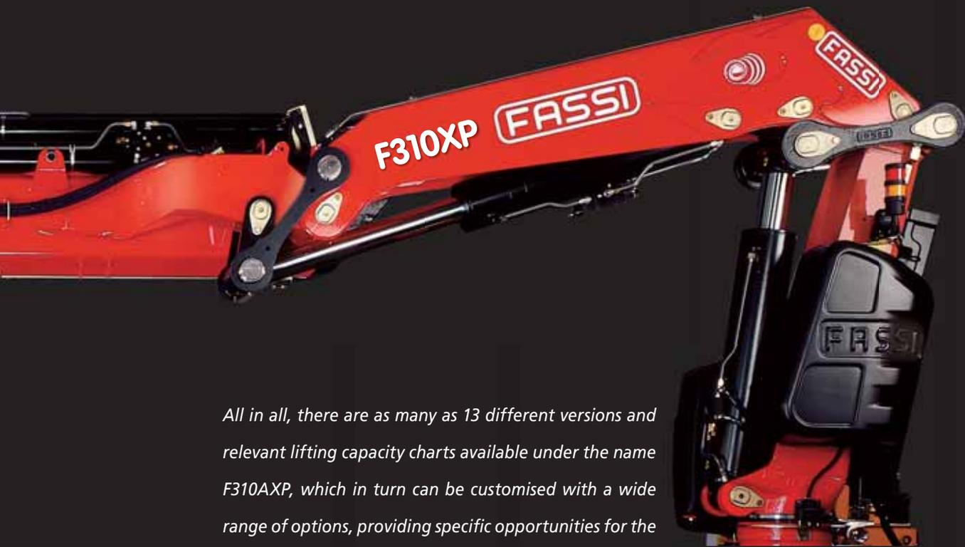
*All in all, there are as many as 13 different versions and relevant lifting capacity charts available under the name F310AXP, which in turn can be customised with a wide range of options, providing specific opportunities for the hydraulic part, articulation of the booms, thermal regulation devices, controls.*
