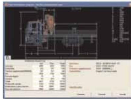
This screen performs an automatic control of weight distribution. If the distribution is suitable, the message CHECKED will appear in red.
