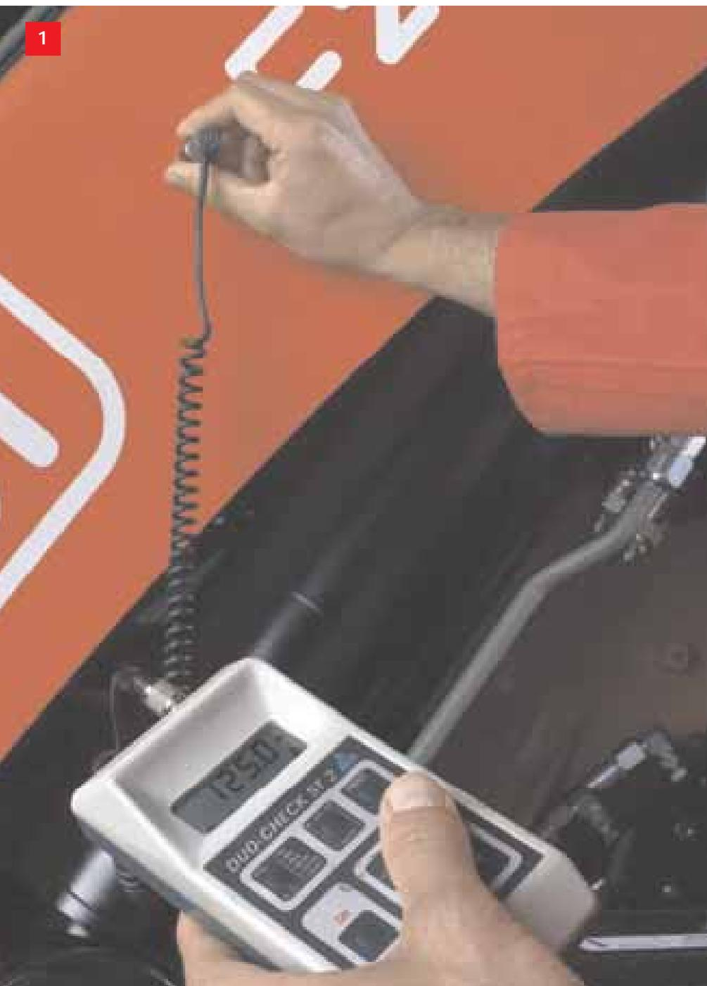
Fassi plants implement a co-ordinated series of controls for final testing of paint quality, including testing of the thickness and quality of the paint layer applied ( photo 1 ) and an abrasion test ( photo 2 ). The aim of these tests is to check that the painting processes comply with those perfected in co-operation with BASF, which involve three essential working phases: phosphodegreasing, application of the epoxy primer and application of the enamel finish (sequence of photographs below).
