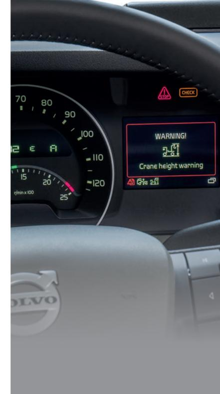
Thanks to the FX-Link, the management of safety messages about the crane's status by the Crane Position Monitoring system can be remotely controlled on the truck's display.
