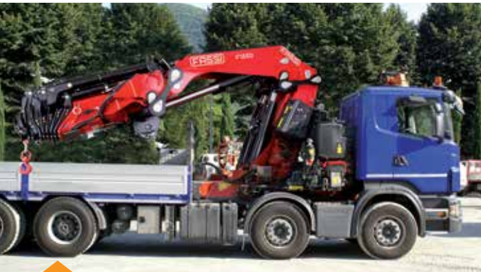
The F1550RA offers a lifting capacity of 123.13 tm
