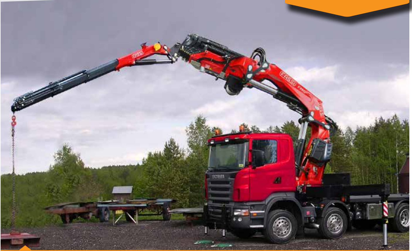
The F990RA in action. The new Fassi crane is equipped with the FX900 electronic system and FX901 panel
