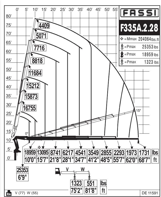
US Dynamic load diagrams calculated, tested and certified to lift the loads at the declared reaches
